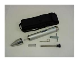
Pilodyn is an easy-to use wood testing instrument. It makes it possible to assess the extent of decay objectively, and to determine the amount of strength loss it has caused! But it can also be used as a general testing instrument for all kind of timber!
